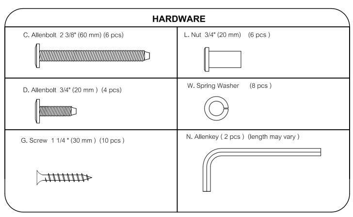
Make sure the bolts are tightly locked against the washers during assembly. (Please add an extra ½ revolution to all the bolts when using spring washer after tightening)
